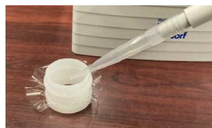
atmospheres are plotted for each element. The results show that the lower energy X-ray (Na, Mg, Al, and Si) are more difficult to detect due to the higher absorption of X-rays by the atmosphere. On the other hand, in a helium atmosphere, the absorption of X-rays is smaller than in atmosphere. For liquid samples that are difficult to keep in a vacuum atmosphere, the sample chamber has been replaced with helium gas for measurement.
