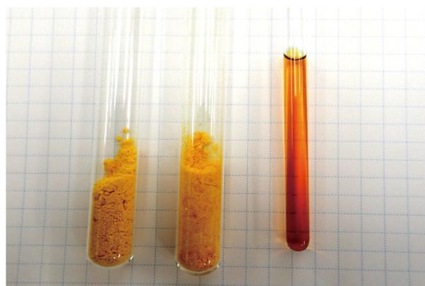
500 mg tungsten complex in 10 mm NMR tubes (left and center).
