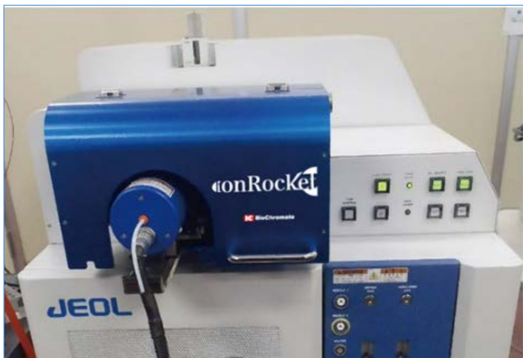
Figure 1. The ionRocket thermal desorption/pyrolysis system mounted on the AccuTOF-DART 4G mass spectrometer
