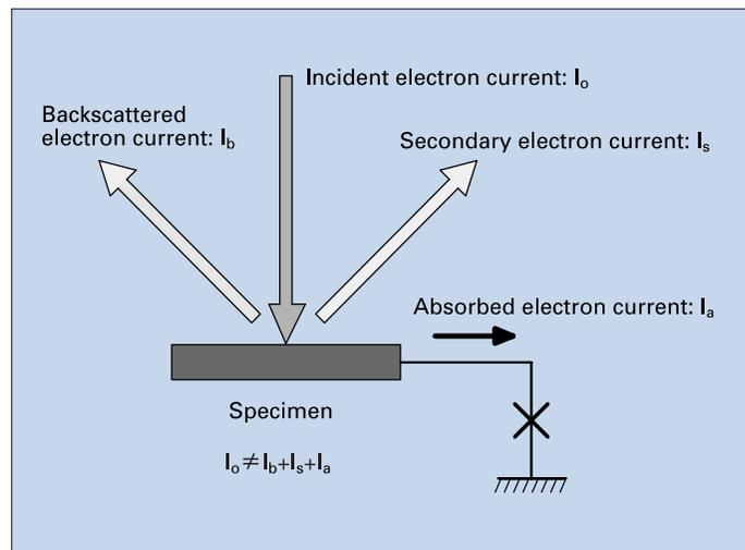
Fig. 39 Electric flow in a nonconductive specimen.
