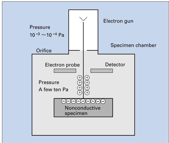
Fig. 44 Schematic diagram illustrating the principle of the LVSEM for observation of nonconductive specimens.
