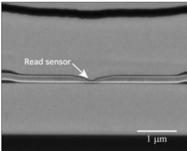
Fig. 17 Example of a backscattered electron image.
