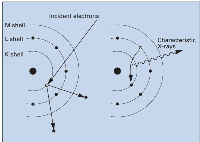
Fig. 49 Principle of the generation of characteristic X-rays.
