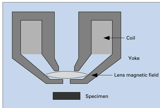
Fig. 34 Construction of the conventional objective lens.
