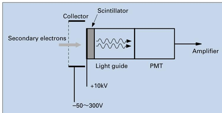
Fig. 6 Construction of the secondary electron detector.
