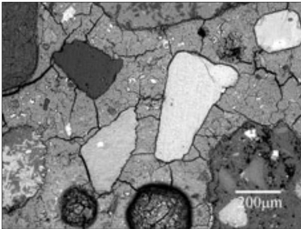
Fig. 47 Observation example of a concrete piece using LVSEM.
