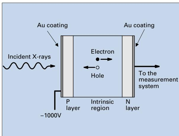
Fig. 50 Construction of the EDS semiconductor detector.
