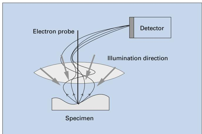
Fig. 26 Illumination effect of a TTL detector.
