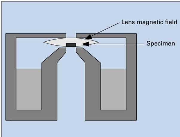
Fig. 35 Construction of the in-lens objective lens.
