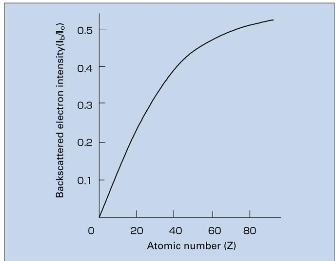
Fig. 16 Atomic number dependence of backscattered electron intensity.
