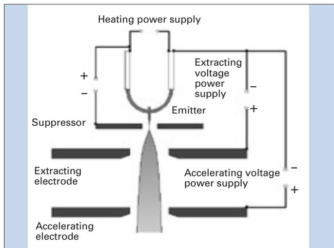
Fig. 31 Construction of the SE gun.
