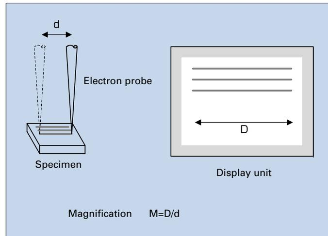
Fig. 7 Concept of SEM magnification.
