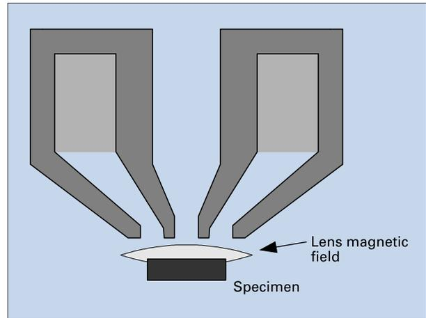
Fig. 36 Construction of the semi-in-lens objective lens.
