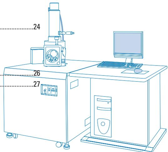
The Scanning Electron Microscope (SEM) is used for observation of specimen surfaces. When the specimen is irradiated with a fine electron probe, secondary electrons are emitted from the specimen surface. Topography of the surface can be observed by two-dimensional scanning of the electron probe over the surface and acquisition of an image from the detected secondary electrons.
