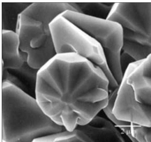
Fig. 15 Secondary electron image of tungsten oxide crystal.
