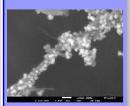
Catalyst particles on carbon nanotube. 3kV mixed SE and BSE image. Sample courtesy of lan Barney, Wright State University.
