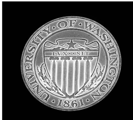
*An etching of the University of Washington seal made with the JEOL direct write e-beam system at [Cornell Nanoscale Science & Technology Facility](#).*
