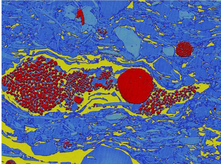
Several energy companies that are investigating alternative sources of fuel oil have turned to JEOL for a new sample preparation solution. Using a process unique to JEOL - an ion beam cross section polisher - they create pristine cross sections of shale for imaging in the SEM.
