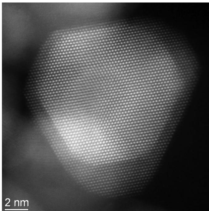
HAADF image of a AuPd core-shell nanoparticle taken on the aberration-corrected JEOL JEM-2200FS at [Oak Ridge National Labs](#). Image courtesy of Miguel Yacamán at UTSA.
