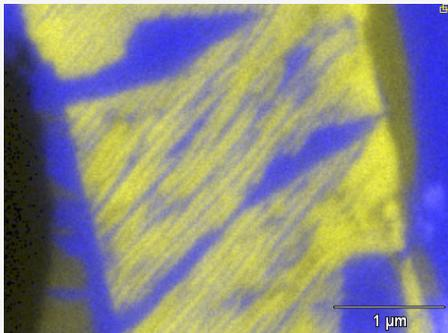
An EDS map of TiO<sub>2</sub> in FeO<sub>x</sub> with <100nm spatial resolution at 30,000X. From the JEOL Analytical Field Emission SEM, the [JSM-7600F](#).
