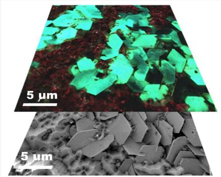
**Aluminum Gallium Nitride SEM image overlaid with ChromaCL image. Performed with JEOL JSM-7600F Analytical Thermal FE SEM.**
