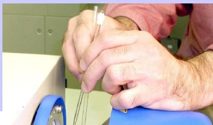
AccuTOF-DART is cutting edge technology for real-time monitoring of chemical reactions, analysis of TLC plates, and characterization of synthetic and natural products. Analyze reaction mixtures by simply dipping a glass rod in the reaction pot
