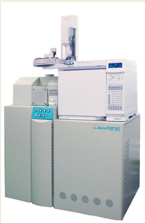
The AccuTOF-GC satisfies both demands for high speed responding to the fast GC method, and for obtaining accurate mass easily.
