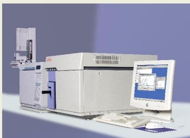
JEOL's GCMate II, a compact, double-focusing, reverse geometry magnetic sector mass spectrometer is explained [here](#).
