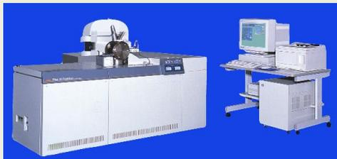
The [MStation™](#) is a fully-automated, high-performance, double-focusing magnetic sector mass spectrometer designed for both high-resolution GC/MS and LC/MS analyses. The MStation is capable of achieving a resolving power of 60,000 or greater at 10% valley.
