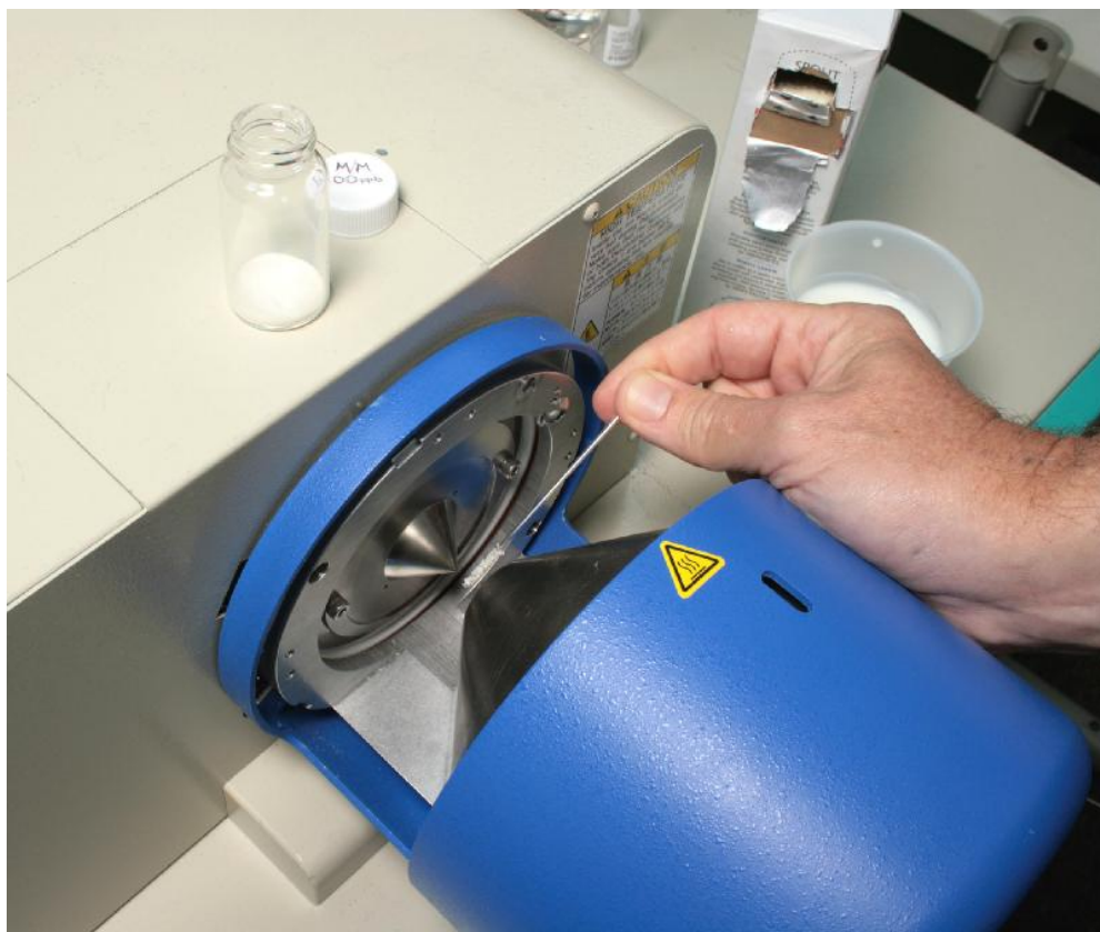
Tartaric acid sampled with a melting point tube
