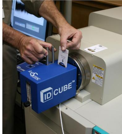
The [ID-Cube](#) enhances the [AccuTOF's](#) performance with all the advantages of DART: no sample prep, no salt interference, and near-instantaneous detection of intact sample on the target screen of an OpenSpot™ Sample Card and insert the card into the slot of the open air ion source for rapid identification.
