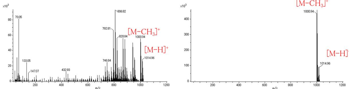
Fig.3 Mass spectrum of Octa(dimethylsiloxy)silsesquioxane by EI (left) and FI (right).
