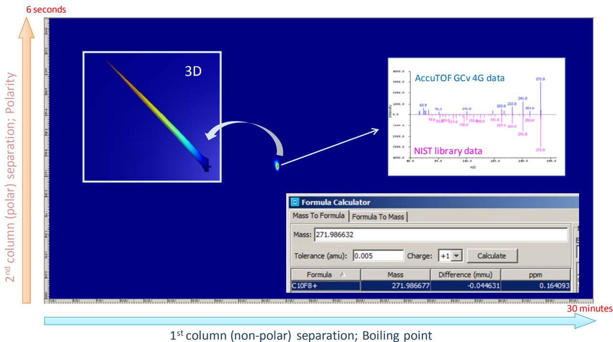
Figure 2. 2-dimensional and 3-dimensional mass chromatograms, library search result and accurate mass measurement results using the OFN 1pg data.
