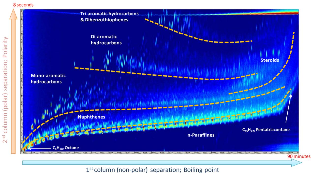
Figure 4. 2-dimensional TIC chromatogram for crude oil (50 Hz data acquisition).
