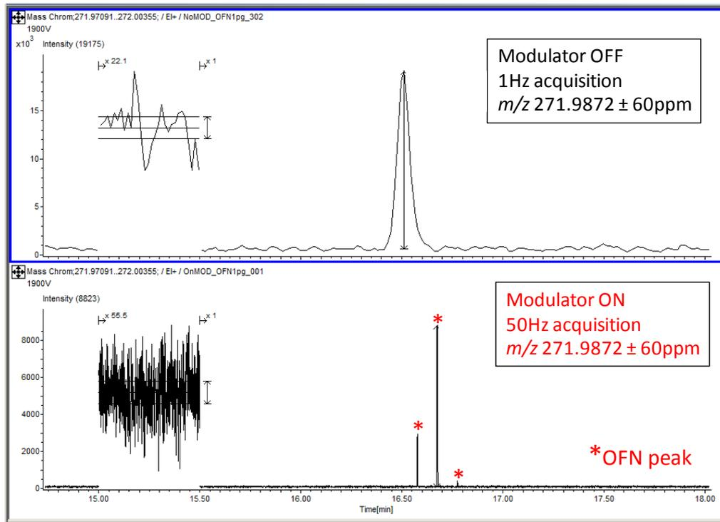
Figure 1. Mass chromatograms of OFN 1pg, Raw data, Mass windows:  $m/z$  271.9872 ± 60ppm
