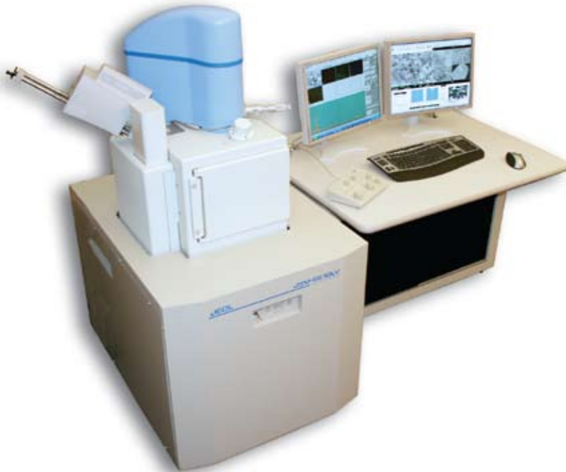
Fig. 5 SEM/EDS systems are used to support scale management programs at Nalco Sugar Land, TX; Naperville, IL; Macae, Brazil; Leiden, The Netherlands; and Aberdeen, UK facilities.
