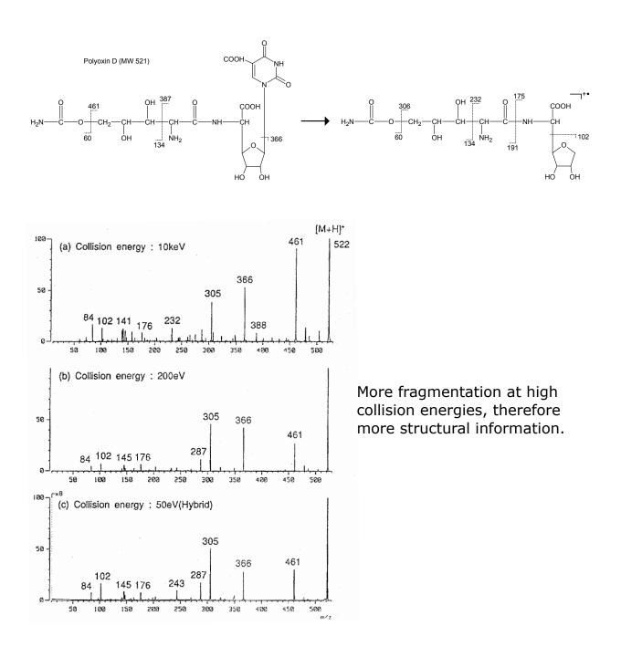
MS/MS of Polyoxin D at Different Collision Energies
