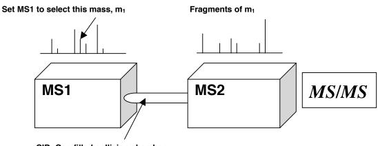
CID: Gas-filled collision chamber. m1 breaks apart to produce fragments
