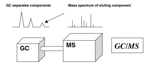
Simple Schematic of a Mass Spectrometer Interfaced to a GC
