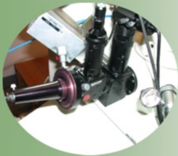
Optical coupling to JEOL 8100/8200 electron probe microanalyzer
