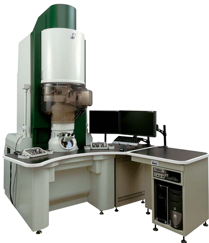
Figure 1. JEOL JEM-ARM200F atomic resolution analytical microscope.
