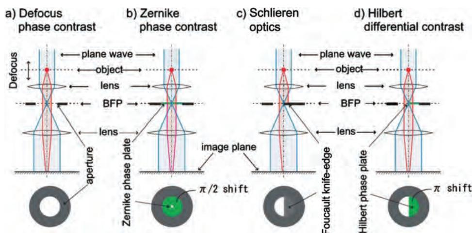
**Figure 1:** Various phase schemes in microscopy. (a) Defocus phase contrast (DPC) by objective lens defocusing and without phase plates. (b) Zernike phase contrast (ZPC) with a Zernike phase plate. (c) Schlieren optics (SO) or singlesideband imaging (SSI) with a Foucault knife-edge. (d) Hilbert differential contrast (HDC) with a Hilbert phase plate [1].
