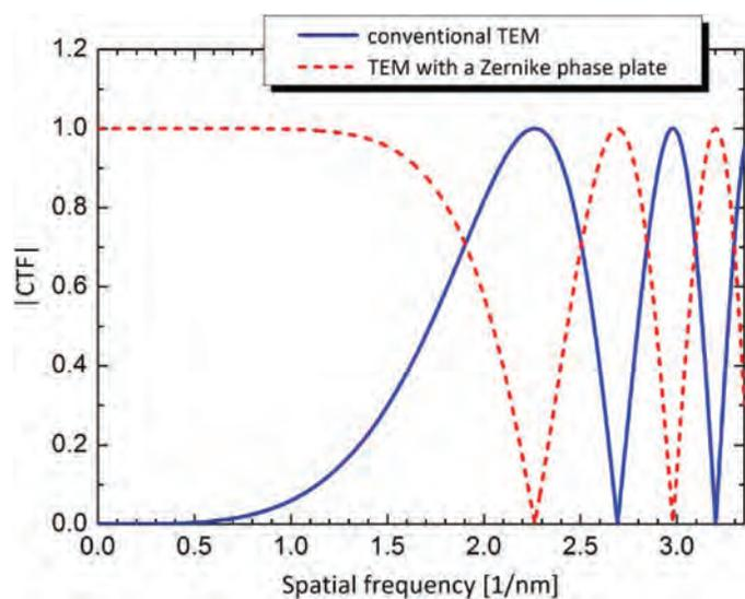
**Figure 2:** Moduli of phase contrast transfer functions (CTFs) without (solid line) and with (dashed line) a Zernike phase plate.  $k_{co}$  is the cut-on frequency of the phase plate determined by the finite size of the central hole of the Zernike phase plate. Parameters for the CTF calculation: defocus 0, spherical aberration 5 mm, accelerating voltage 300 kV.
