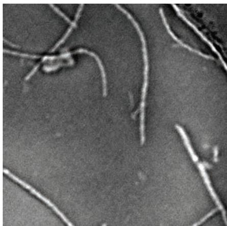
Elk fibrils imaged at liquid nitrogen temperature (left) in standard bright field TEM imaging and (right) with hole-free phase plate. Sample courtesy of H Young and JP Glaves (biochemistry, University of Alberta), data was taken by Julie Qian, NINT Electron Microscopy.
