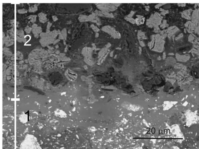
**Figure 4.** Backscattered-electron image showing the diffusion of lead soaps formed in the lower lead white paint (layer 1), which migrate into the upper Emerald-green-containing paint layer (layer 2). Sample removed from “Old-Holland table” (late-18th century) from “de Markiezenhof,” Bergen op Zoom.
