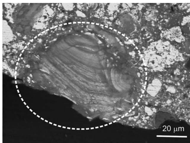
**Figure 7.** Backscattered-electron image showing lead soap aggregates in a more developed stage with lead carbonate-containing mineralization bands inside (indicated with dotted line). Sample from Christiaan van Couwenbergh's *Herald* (southwest) (1651), oil on canvas, Oranjezaal, Royal Palace Huis ten Bosch, The Hague.
