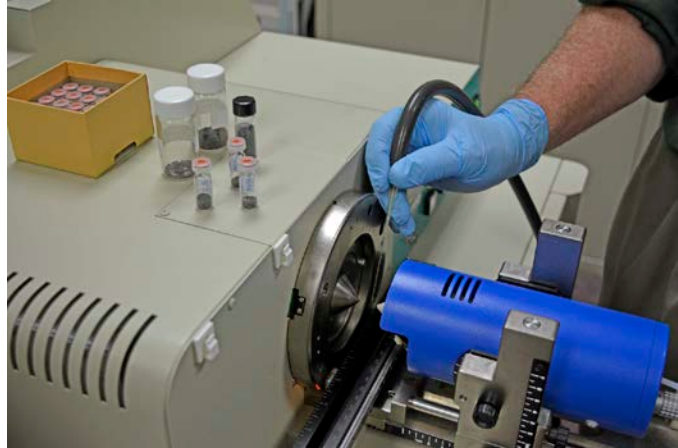
Figure 2. AccuTOF-DART analysis of a smokeless powder particle.
