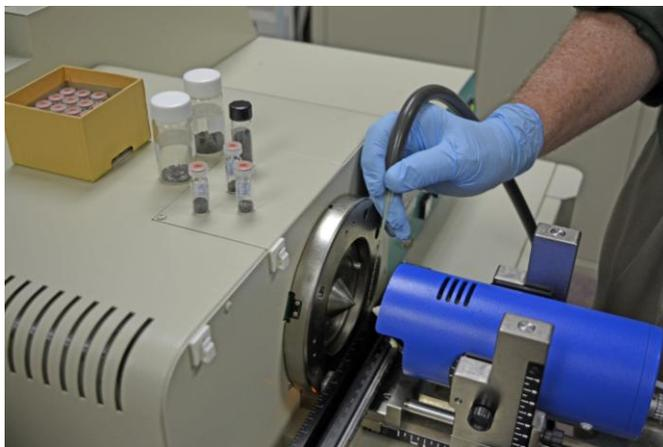
*Figure 2. AccuTOF-DART analysis of a smokeless powder particle.*
