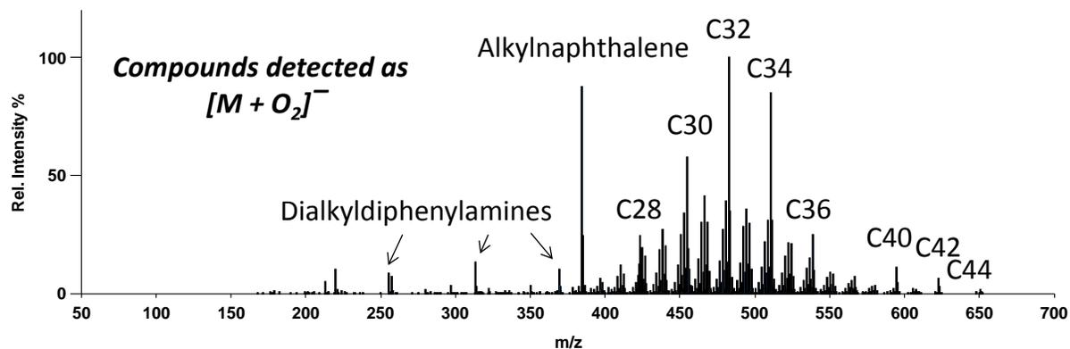
Figure 2. Negative-ion O<sub>2</sub><sup>-•</sup> attachment DART mass spectrum of the motor oil from Figure 1, showing the base oil components including C24-C44 alkanes and an alkyl naphthalene.
