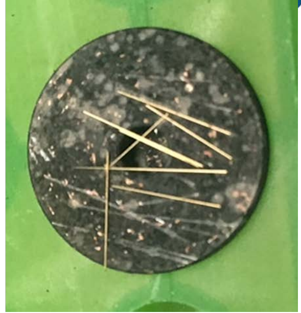
Figure 2. Segments of welding wire placed on the surface of the copper sample stages for the IonRocket. The left figure shows the wires placed on a fresh, clean sample stage, and the right side shows wire segments on the surface of a copper sample stage that was oxidized after heating to 600°C.
