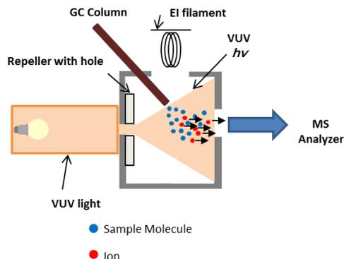
Figure 2. Schematic of the PI ion chamber.
