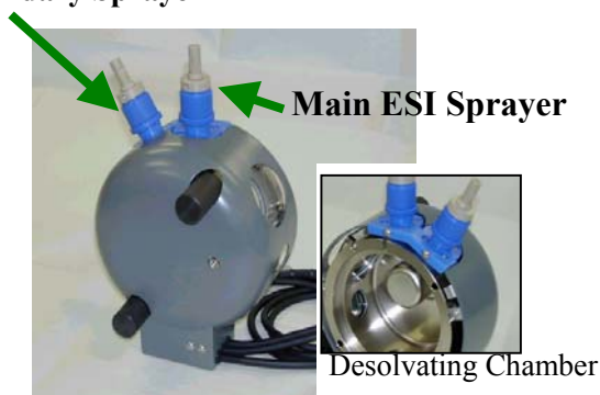
Figure 1. Dual ESI Ion Source
