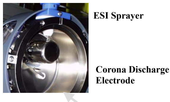
Figure 2. Corona ESI Ion Source
