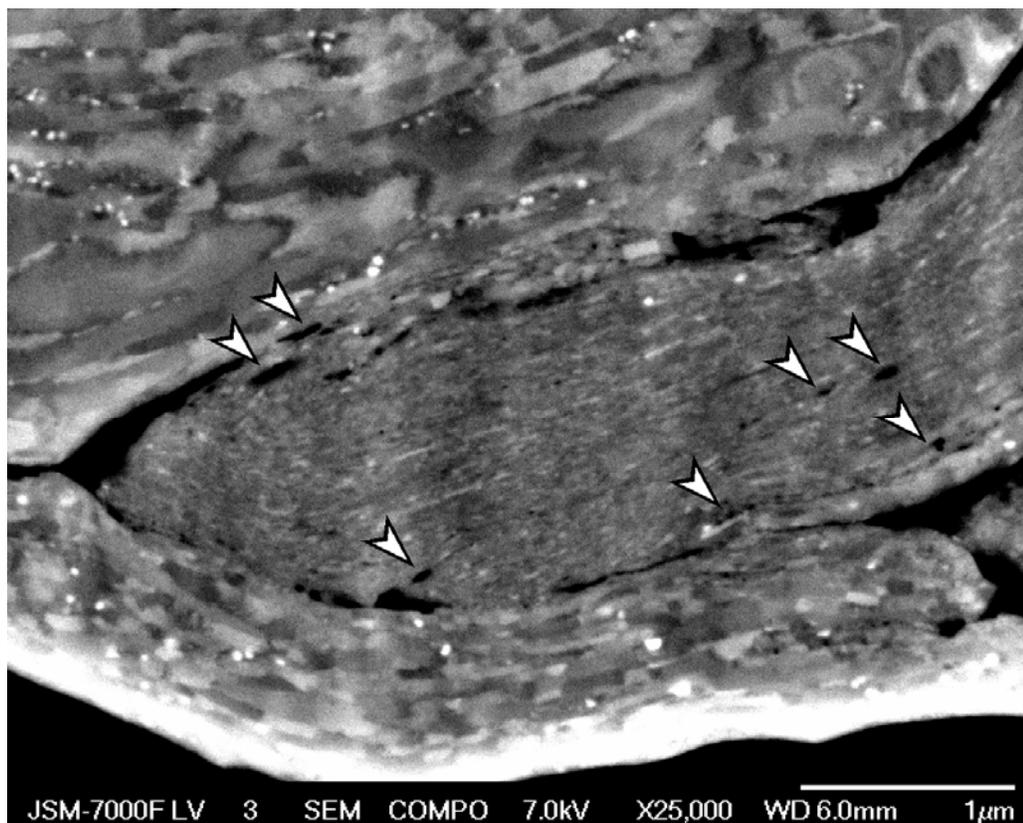
Fig. 2. Backscattered electron image (25,000x) of cryomilled Al powder cross-sectioned by the CP showing both nanocrystalline and coarse-grain structures with arrows indicating submicron voids.
