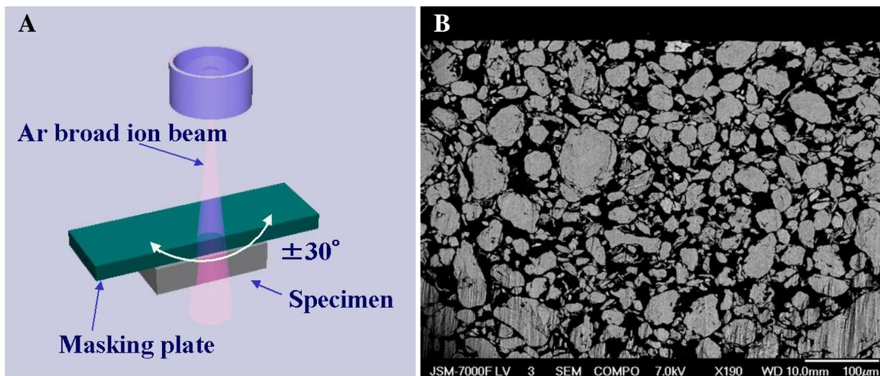
Fig. 1. (A) Schematic of general operation of a CP. (B) Backscattered electron image (190x) of CP prepared powders.
