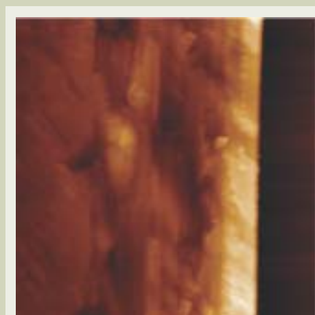
Fig. 7 AFM image of a cross section of a multi-layer optical film. (scan size : 4\text{ }\mu\text{m} \times 4\text{ }\mu\text{m} )
