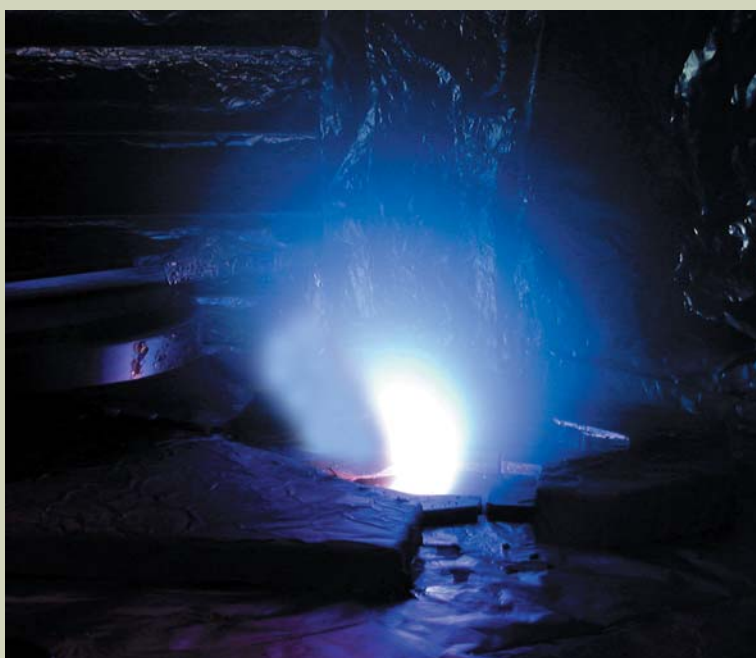
Fig. 3. Plasma discharge in \text{Ta}_2\text{O}_5 deposition process.
