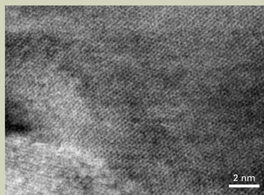
Fig. 6. High-resolution STEM image. Specimen: Silicon (111). A lattice fringe of 0.192 nm can be clearly observed.
