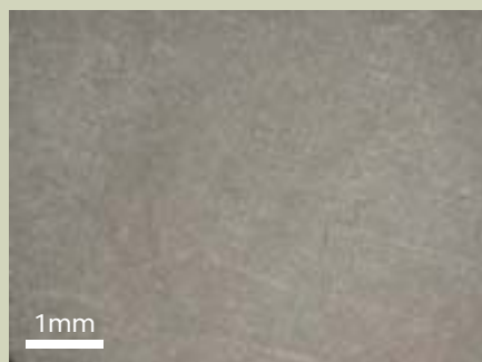
Fig. 2. Photograph of the central of the electrode observed using the optical microscope (The surface color is black and the shape changes are not observed).
