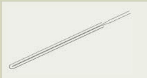
Fig. 1. Pasteur pipette for sample preparation.
