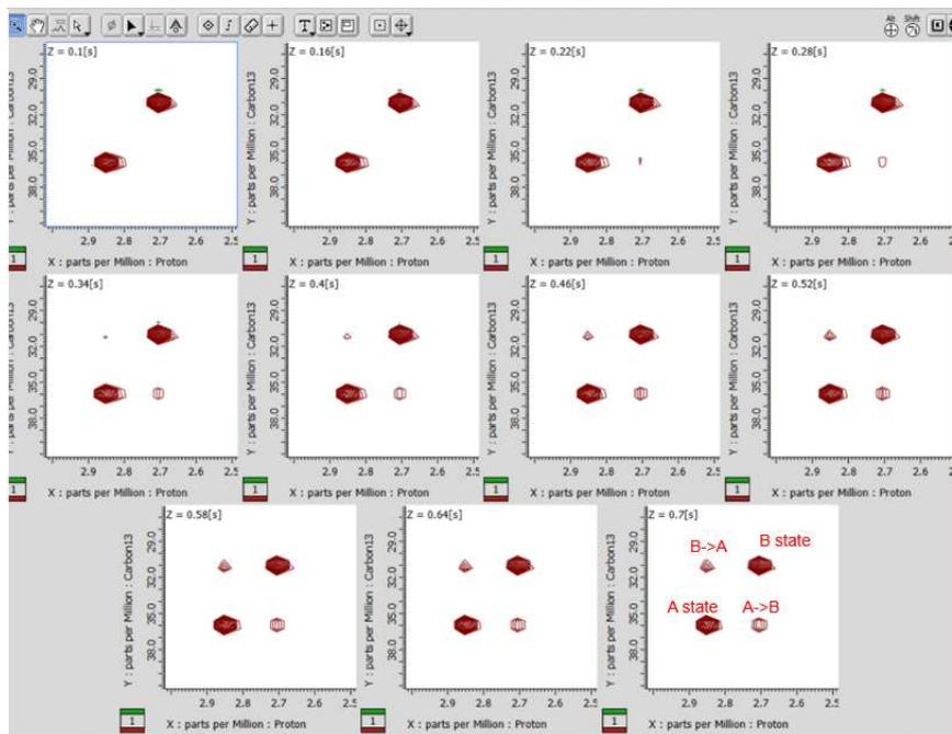
Fig 3:  $^1\text{H}$ - $^{13}\text{C}$  ZZ exchange experiment for DMF in  $\text{DMSO-d}_6$ . The 2D experiment was executed as array measurement for the acquisition parameter "mixing time". The result is a single pseudo-3D data file with the recorded values of mixing time on the Z-axis
