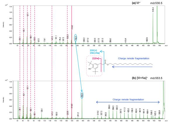
Figure 2. Product ion spectra of IRGANOX 1076 with different ion species. (a) m/z 530 M<sup>+\*</sup>. (b) m/z 553 [M+Na]<sup>+</sup>.
