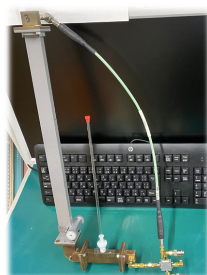
Fig.1 (a) A drawing of transmit absorption measurement. (b) An example of transmission ESR/FMR measuring device using a wave guide.
