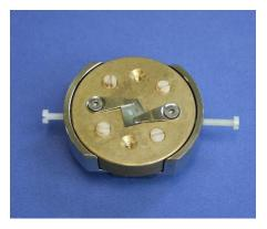
Figure 2: Polymer screws isolate cryo-stub from holder
