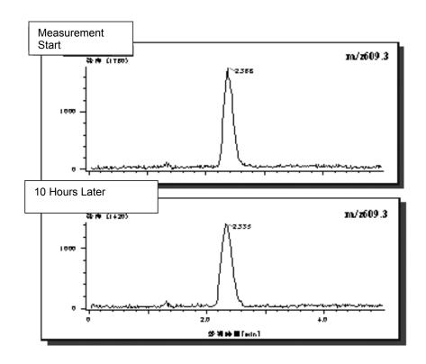
Figure 3. Intensity Change of Reserpine when Phosphate Buffer is Used (Top: At start time; Bottom: Ten hours later)
