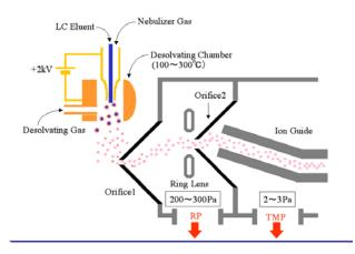
Figure 1. Schematic Diagram of ESI Source and API Interface
