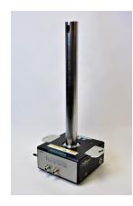
The new 2mm Magic Angle Spinning (MAS) Probe is well suited for both materials and biosolids NMR.
