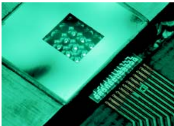
A micro-optical stack containing a 4x4 array of a microlens chip on top of a micro-shutter chip. Control signals for the shutters are fed through the electrical connections seen at the front of the image.
