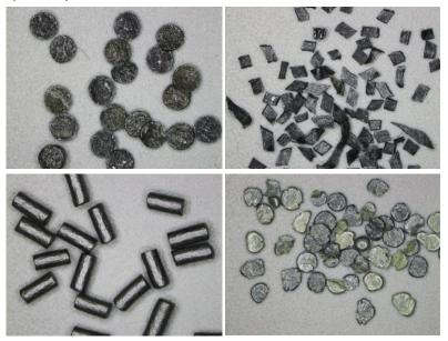
Figure 1. Several smokeless powders viewed under an optical microscope.
