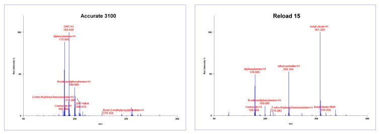
Figure 3. (a) AccuTOF-DART mass spectrum of an Accurate 3100 smokeless powder particle; (b) AccuTOF-DART mass spectrum of a Reload 15 particle.
