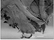
Scanning electron microscope (SEM) images of the apex of a triangular piece of filter paper used for PaperSpray ionization. The secondary electron detector images were obtained for gold sputter-coated paper at 3 kV with the JEOL IT100 Scanning Electron Microscope.
