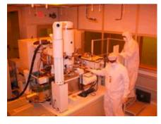
Georgia Tech's Microelectronics Research Center (MiRC) currently operates a JEOL JBX-9300FS 100kV electron beam lithography system. The JBX-9300FS features a spot beam, vector scan, a step and repeat stage, and is capable of varying the beam size widely. Its dynamic correction system eliminates defocusing resulting from beam deflection. The system is versatile in exploring new frontiers in
