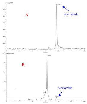
Fig.1 Mass chromatograms of acrylamide extracted from French fry sample. (A) high resolution, (B) low resolution
