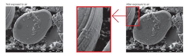
Fig. 3: LiCoO<sub>2</sub> particles in positive electrode before and after air exposure. Clearly, air exposure introduces various artifacts affiliated with specimen reactivity with atmospheric oxygen.
