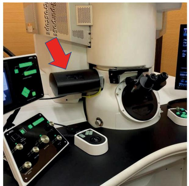
A camera for acquiring diffraction patterns is built in the area indicated by the arrow.
