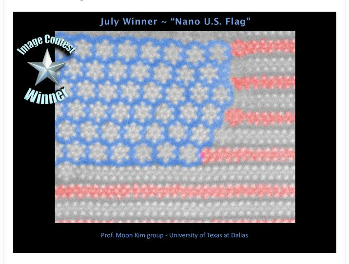
Congratulations to <u>Dr. Moon Kim'</u>s group, University of Texas at Dallas for this ARM200F TEM image: "Atomic scale Mo6Te6 nanowires transformed from its parent MoTe2 2D layers. Each nanowire, 0.8 nanometers in diameter, consists of six molybdenum (Mo) atoms surrounded by six tellurium (Te) atoms." <u>More about this image</u>>>>
