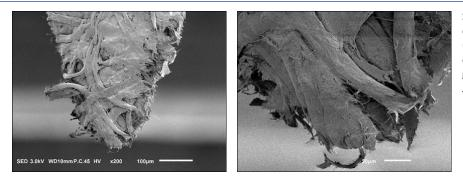
Scanning electron microscope (SEM) images of the apex of a triangular piece of filter paper used for PaperSpray ionization. The secondary electron detector images were obtained for gold sputter-coated paper at 3 kV with the JEOL IT100 Scanning Electron Microscope.
