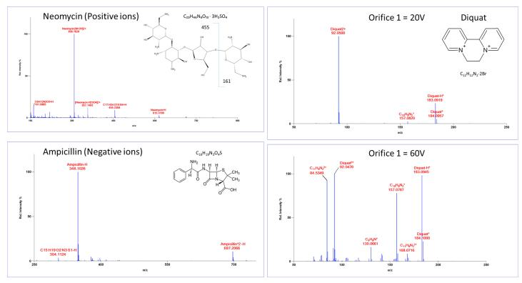
The positive-ion PaperSpray mass spectrum of neomycin with an orifice 1 voltage of 25V (top) shows peaks for both double-charge and single-charge neomycin and smaller peaks for neomycin sulfate and fragments resulting from loss of an aminoglycoside. The negative-ion PaperSpray mass spectrum for ampicillin show deprotonated ampicillin and dimer and a small fragment corresponding to loss of CO<sub>2</sub>.
