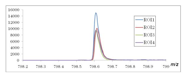
Figure 2. Mass spectra of ROI 1 - 4 at m/z 798
