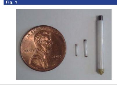
A picture of three MAS rotors used for this study in a comparison with a US one-cent coin. (Left) JEOL 0.75-mm rotor, (middle) JEOL 1-mm rotor, and (right) Varian 2.5-mm rotor.
