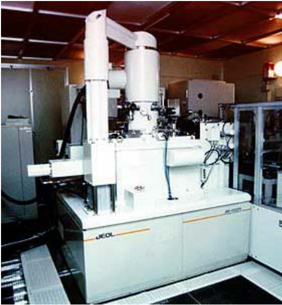
Fig. 1. First JBX-9300FS was installed at NEC Sagamihara plant in Japan. EB system is combined with in-line developer.
