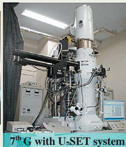
Fig. 3 History of development of JEOL cryo-electron microscopes with helium stage. From the first generation cryo-EM to the seventh generation one.
