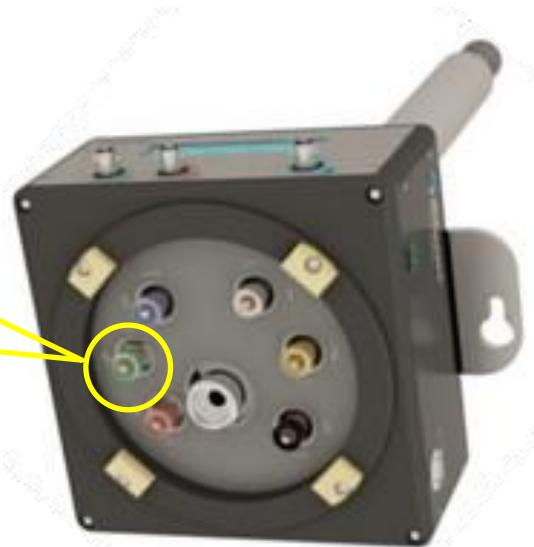
AutoTune Extension Automatically switches between HX & HFX modes
