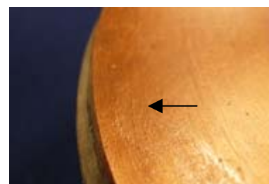
Fig. 1 Organic contamination on metal surface
